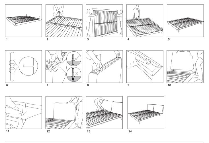
To separate the base: If the base does not fit through the front door, the following steps need to be undertaken to split the King or Queen sized frame into two pieces.
